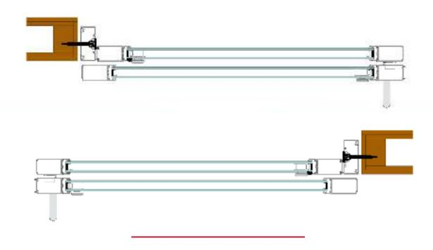
Closure detail with integrated leading edge seals
